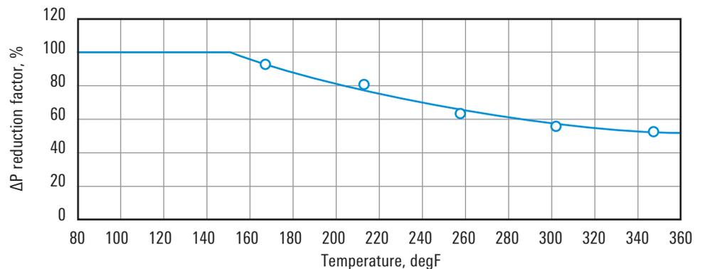
*This elastomer-temperature capability curve highlights the percentage of maximum pressure differential that can be expected based on circulating temperature.*
